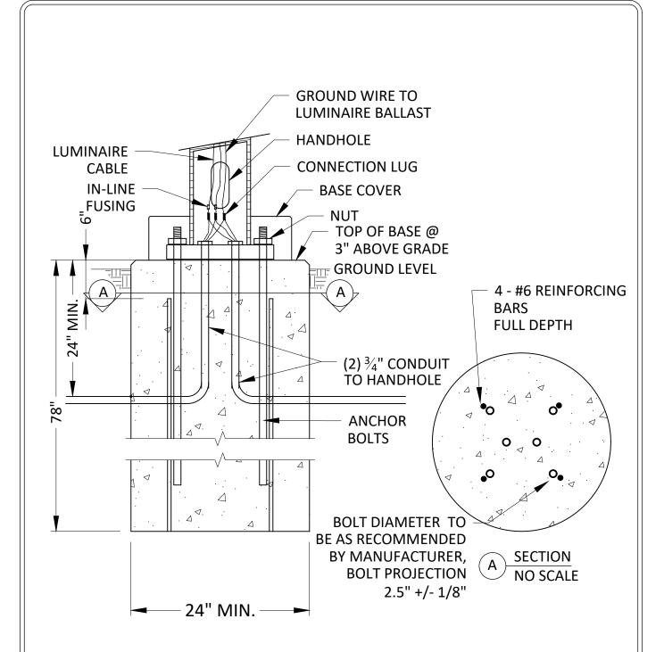
NOTES: 1. 5/8" X 10'-0" GROUND ROD TO BE LOCATED IN HANDHOLE ADJACENT TO BASE.
